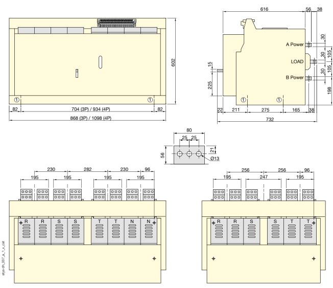
1. Fixing hole base: Ø13 mm
